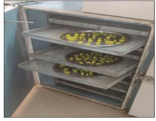
Plate 5: Grapes were kept inside the tray dryer for drying for 8h
