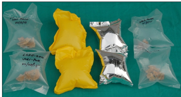
Fig. 1. Gum karaya samples packed in LDPE, HDPE, ACP and PP film with nitrogen filling
